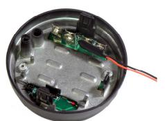
batteries from the lock keypad then plug the white end of the JumpBox cable into any one of the 9-volt battery snap connectors inside the keypad in place of the battery (see images to left).
