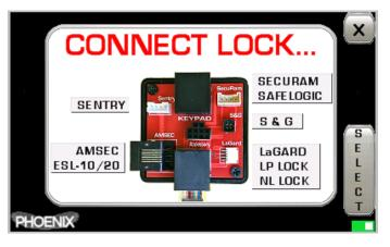
attached lock. If the tool is unable to accurately detect or identify the connected lock (possibly due to a damaged cable or lock electronics) then you can tap the vertical **SELECT** button on the right side of the screen to manually select the type of lock you're wanting to connect to.
