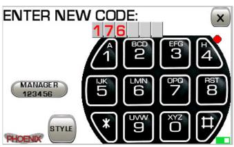
aborts the entry procedure and returns to the previous menu. During *Lock Servicing*, the Phoenix keeps a record of any manager or user codes programmed in the lock and places a handy quick entry button on the left of the keypad showing the user type and current code. Tap the quick entry button to automatically enter the code in the keypad.
