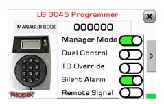
current settings in the 3045 Programmer Menu. If the displayed Manager Code is incorrect, tap the code to update it. Use the RIGHT ARROW to transition to the 2<sup>nd</sup> menu then tap SEND to transfer the indicated settings to the lock.
