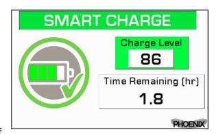
charge completion. Once this occurs, simply unplug the charger and the Phoenix will power itself down automatically. In order to see the benefits of the Smart Charge feature it is important that you remove the charger from the Phoenix in a timely manner once a 100% charge level is reached. The included charger will continue charging the internal battery module tool as long as it remains connected to the Phoenix. *The only way to cease the charge is by disconnecting the charger from the tool.*
