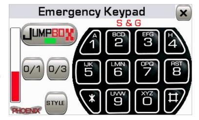
rotating motor will show a huge a large red spike immediately. The **JumpBox** circuit is accessible from inside the **Emergency Keypad** by tapping the **JumpBox** button. The GREEN will show when the JumpBox circuit is active. On S&G locks, two additional buttons are shown that allow sending the special [0/1] and [0/3] button combinations used with MRC codes.
