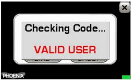
Phoenix will begin to confirm the supplied code. If the code is determined valid then the Phoenix assumes that the problem must be mechanical in nature and will use its built-in JumpBox circuit along with its pre-programmed diagnostic routines to repair and open the lock. Examples of these issues include stuck solenoids, stalled bolts and cross-threaded drive nuts. In many of these cases the lock can be re-used after repair.
